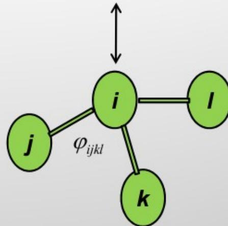
By definition, from the force field parameter and documentation, the first atom listed is the central atom. Therefore just like a normal torsion, the angle of interest is between the plane defined of particle  $ijk$  to that of the plane defined by particle  $jkl$ . This is only used for special situations.
